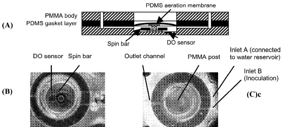
Figure 1: A – Schematic longitudinal section of the microbio-reactor; B – Photograph of the empty chamber of the reactor. The spin bar in the center and the fluorescent sensor for DO (black spot) are visible; C – Photograph of the chamber at the end of the run. Turbidity of the cell culture obscures the spin bar and the DO sensor.
