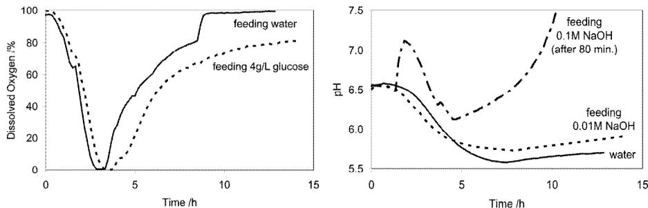
Figure 3: (left) DO for one batch and one fed-batch fermentation run with glucose in the microbioreactor; (right) pH for one batch and two fermentation runs feeding base solution. For the 0.1M NaOH solution, the feeding started at 80 min.
