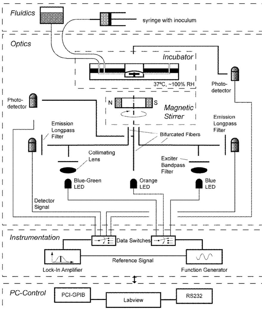
Figure 2: Schematic of the experimental set-up with the instrumentation, the optics, the magnetic stirring, the incubator chamber and the fluidics for reagent feed and inoculation (syringe not attached during run).
