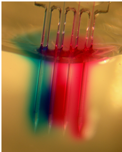
Figure 2. Photograph of a microneedle array inserted into a 8% (w/w) gelatin matrix and dispensing colored solutions through the needles.
