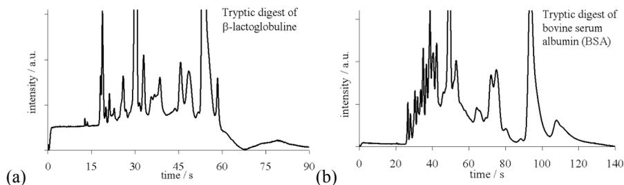
Figure 3. Separation of FITC-labeled tryptic digest of (a)  $\beta$ -lactoglobuline and (b) BSA in ORMOCOMP<sup>®</sup> microchannel of  $50 \mu m \times 28 \mu m$  ( $w \times h$ ). The electric field strength was (a) 700 V/cm or (b) 500 V/cm, other conditions as per Fig. 1b.
