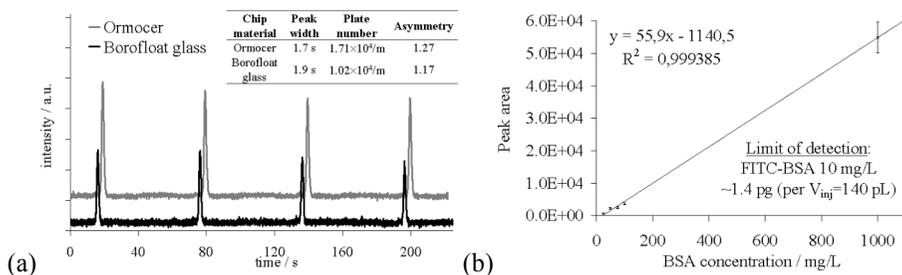
Figure 2. (a) Repeated injections of 1 mg/mL FITC-BSA on ORMOCOMP<sup>®</sup> and Borofloat<sup>®</sup> microchannels (both  $50 \mu\text{m} \times 20 \mu\text{m}$ ,  $w \times h$ ). Separation conditions were as per Fig. 1b. (b) Calibration curve of FITC-BSA between 0.01 and 1.0  $\mu\text{g}/\text{mL}$ .
