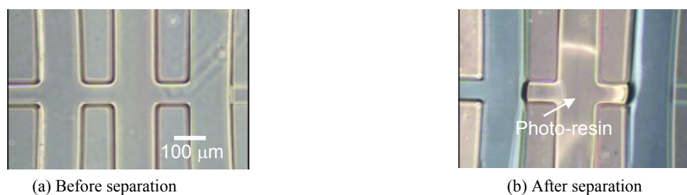
Figure 6: Separation of chambers by in-situ photopolymerization
