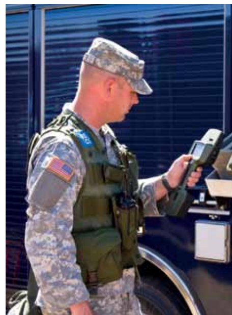
The aptly-named Fido handheld device can detect explosives vapours at levels that almost match a sniffer dog's nose
