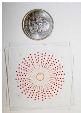
Figure 1. Bright field image of the rotational SlipChip after slipping to form isolated compartments, shown next to a U.S. quarter.
