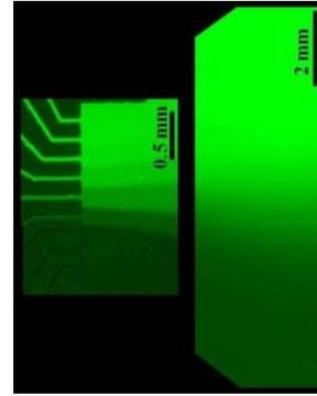
Figure 2: FITC-dex concentration gradient. Top views at the end of the mixer channel network and the chamber entrance.
