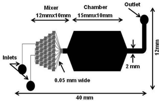
Figure 1: Scheme of the microfluidic device.
