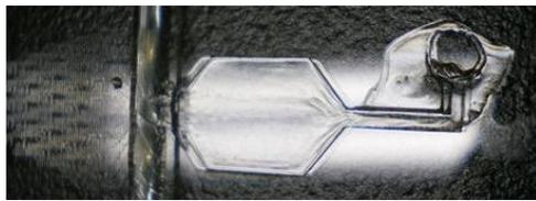
Figure 3: PEG hydrogel after UV polymerization. View with PDMS layer partially removed.
