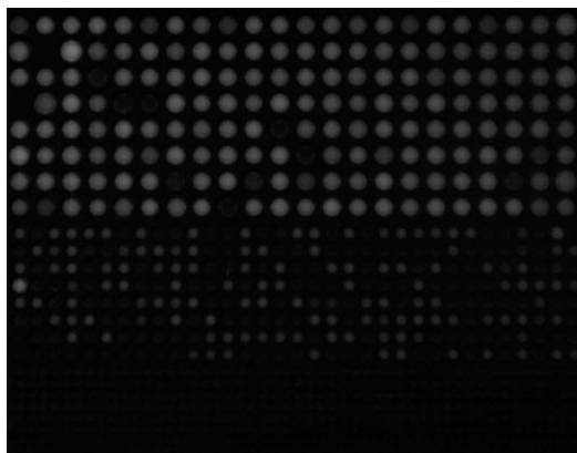
Figure 3. End-point fluorescent image of multi-volume digital PCR assay. Concentration calculated from Poisson equation is 1.9 \times 10^4 molecules/mL.
