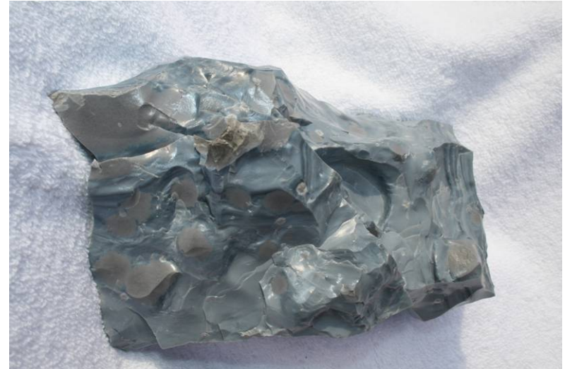
Borosilicate glass incorporating Surrogates of Magnox Sludge and Plutonium Contaminated Waste
