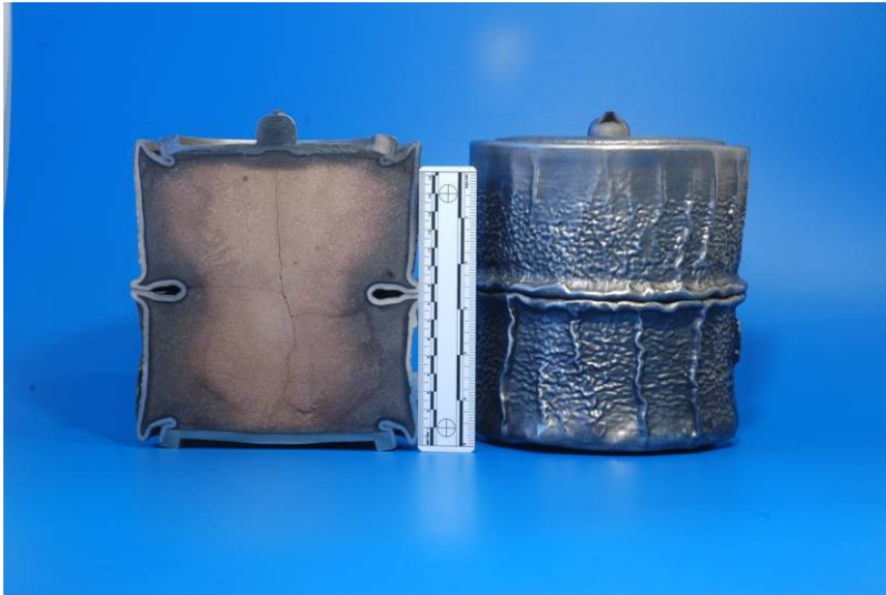
Ceramic from Magnox Sludge Surrogate - magnesium silicates and titanates
