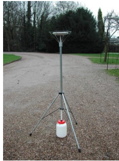
Dry 'Frisbee' deposit gauge (substantial improvement on BS 1747 Part 1 Deposit Gauge)
