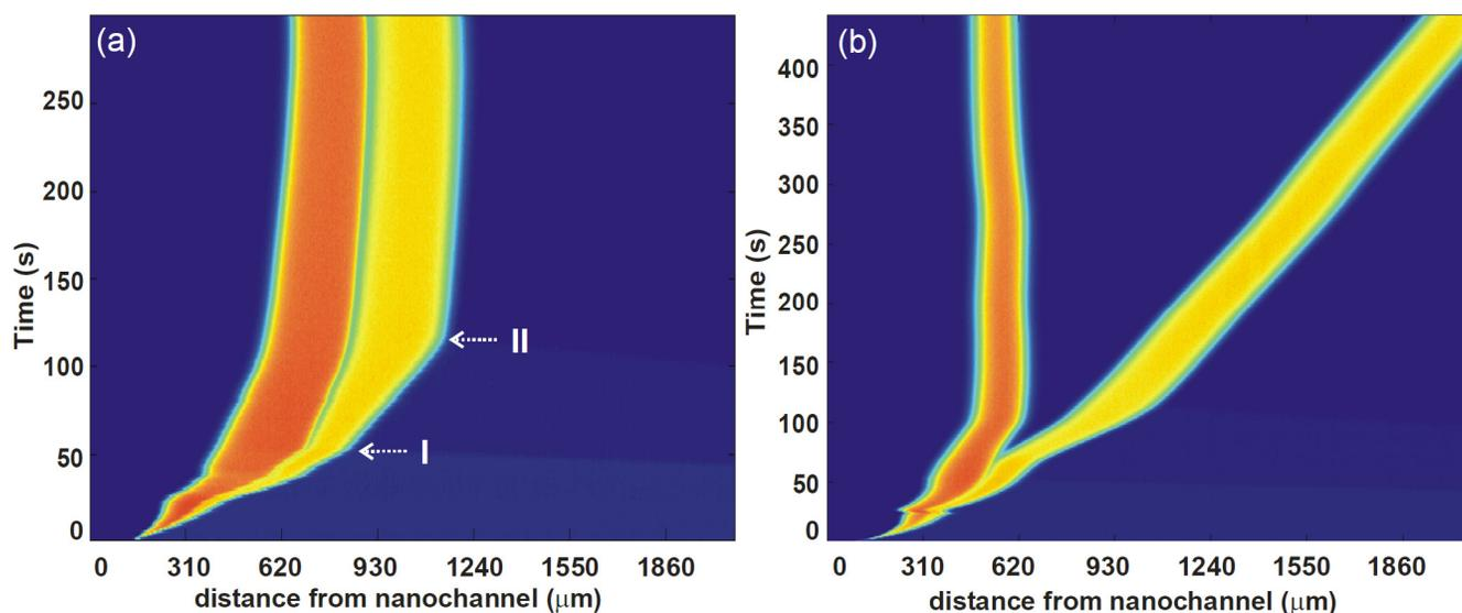
Figure 2: Spatiotemporal plots of dzITP separations. a) Discrete injection of fluorescein and 6-carboxyfluorescein. Arrows I and II indicate exhaustion of fluorescein and 6-carboxyfluorescein respectively. d) Discrete injection of fluorescein and 6-carboxyfluorescein combined with a continuous injection of acetate.
