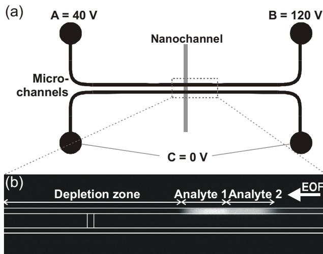
Figure 1. a) Schematic representation of the chip layout, showing two microchannels connected by a nanochannel, and an example of voltages during three-point voltage-actuation. b) Example of dzITP separated zones at the border of a depletion zone. Micro- and nanochannels have been indicated by lines that were drawn upon the photomicrograph
