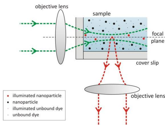
Figure 1: Illustration of the cross-sectional side view of the excitation (green) and fluorescence (red) light path in light sheet illumination.
