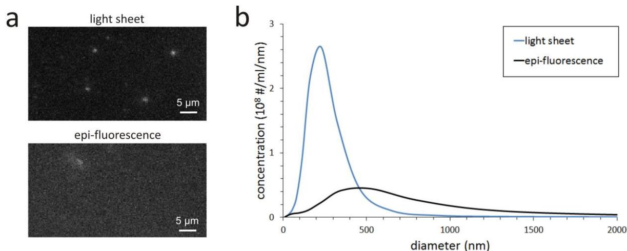
Figure 4: fSPT size and concentration measurements were performed on cell-derived MVs in cell culture medium. (a) The MVs are clearly visible when using light sheet illumination, while only a few MVs are visible for epi-fluorescence illumination due to the much higher background fluorescence. (b) The number concentration is underestimated and biased towards larger MVs for epi-fluorescence illumination versus sheet illumination.
