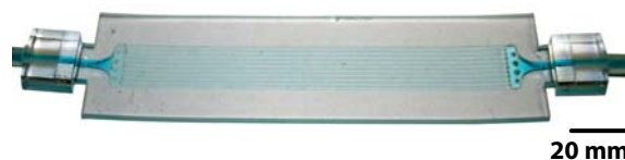
Figure 3: Simplified evaluation model used for the analysis of the cell free blood plasma layer. In this image the simplified EM is filled with dyed water.
