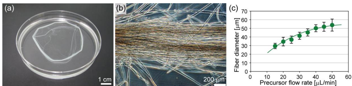
Figure 3: (a, b) A bundle of the obtained fiber with diameter of ~20 \mu\text{m} and a total length of ~200 m. (c) Relation between the widths of the fiber and the total flow rate of the precursor solutions.
