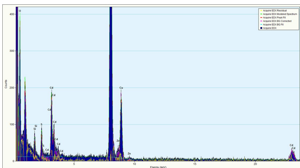
Fig. S2. EDX of CdS:Zn synthesized with 0.2 mmol of Zn(OAc) 2 .
