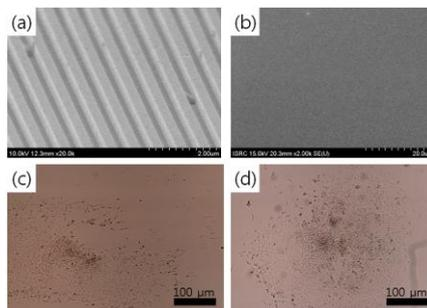
*Figure 2. (a) SEM image of PUA 350nm line structures (spacing of 350 nm, height of 500 nm). (b) SEM image of PUA flat substrate. (c) Bright-field image of hESCs on 350nm PUA line structures. (d) Bright-field image of hESCs on PUA flat substrate.*
