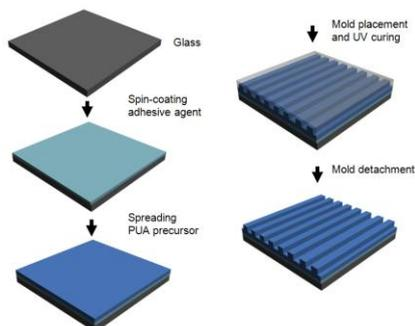
Figure 1. A schematic illustration for the fabrication of PUA nano structures by UV-assisted capillary force lithography (CFL)
