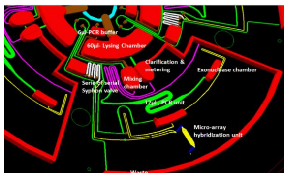
Figure 1. Microfluidic design of integrated CD Lab
