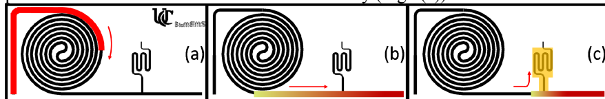
Figure 1. Schematic diagram outlining the function of the biochip with integrated dynamic separation and immunoassay: (a) Blood sample loaded into long channel; (b) Blood sample at the end of long channel using dynamic flow with a gradient of
