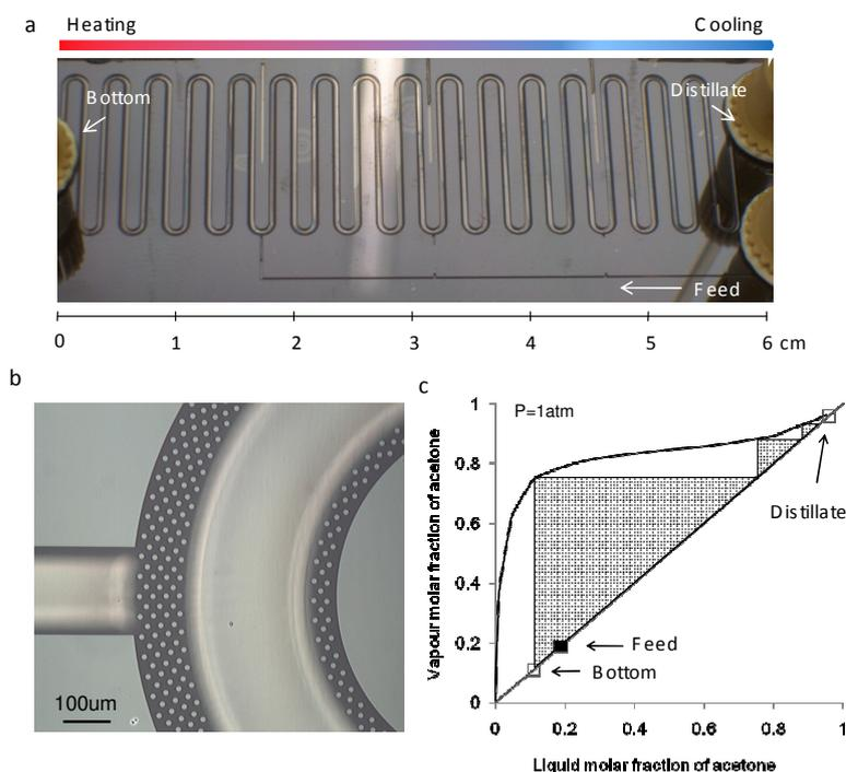
Figure 2: Characteristics of the microscale distillation chip: (a) chip configuration, (b) micro-pillars at the feed location and (c) performance of a 19 mol% acetone-water mixture separation
