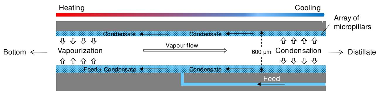
Figure 1: Operating principle of the microdistillation chip illustrated at the feed location
