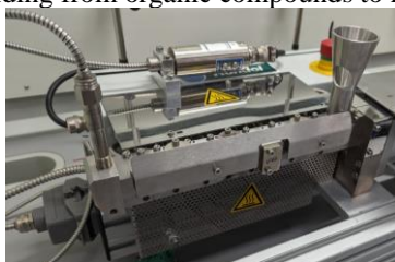
Figure: Twin-screw extruder employed in the continuous, solvent-free synthesis of organic and coordination compounds.
