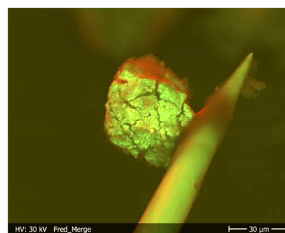
Figure 1: SEM image of a hot particle from the Chernobyl cooling pond fixed to a tungsten tip. Green: BSE image; Red: SE image.
