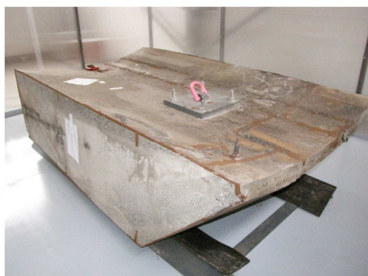
Figure 1: Biological shielding of the VVER 440 type reactor (NPP Greifswald, 5 th block)
