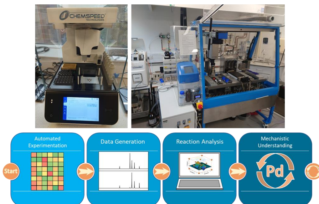
Figure 1 Top: Image of the Chemspeed automation platform and Crystal Powderdose used for catalytic reaction screening and optimisation of reactions for mechanistic insights. Bottom: Workflow procedure from automated experimentation, large data generation, and reaction analysis for greater understanding of palladium catalysed reactions.
