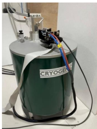
Figure 1 Cryogen-free magnet with MAS probe inside.
