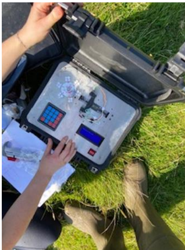
Figure 2. Demonstrating the portable phosphate analyser which uses centrifugal microfluidics, in a
