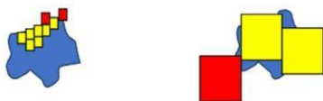
Figure 2: Impact of “pixel to particle image size” ratio on quality of defined shape. Yellow squares represent pixels selected to define a shape; red squares are pixels that are de-selected.
