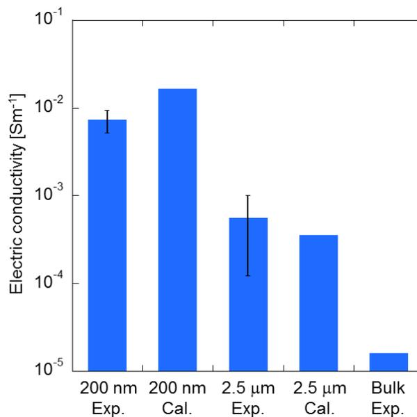
Figure 5. Electric conductivity of water in extended nanospaces and microspaces and bulk. Experimental results were compared to calculated results.
