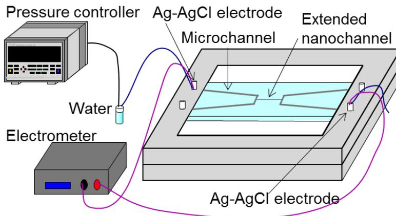
Figure 1. Schematic illustrations of experimental setup for conductivity measurements using a streaming potential/current method.
