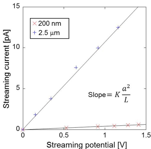
Figure 4. Relationship between streaming potential and current in different channel diameter  $a$ . Its slope is a function of conductivity  $K$ ,  $a$ , channel length  $L$ .
