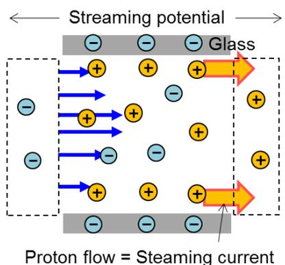
Figure 2. Principle of streaming potential/current by pressure-driven flow.
