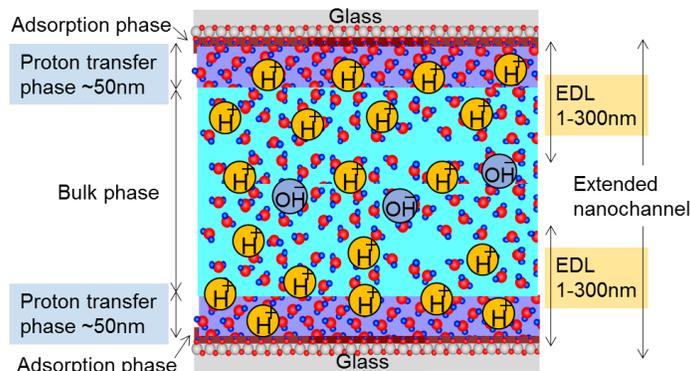
Figure 6. Three-phase model and EDL model in extended nanopspaces discussed in this study.
