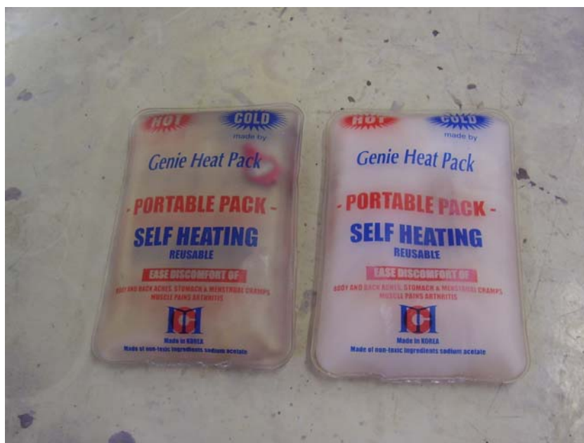
Figure 4. Photo of two commercial sodium acetate portable heating packs, before and after setting off the crystallisation reaction.
