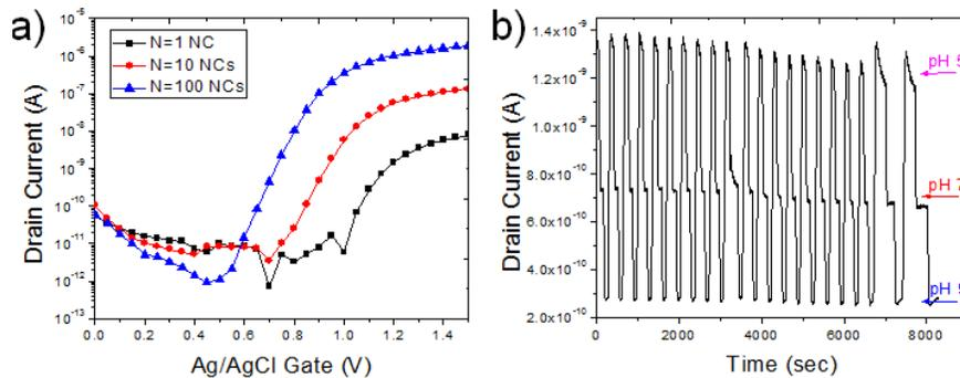
Figure 3: Comparison of device characteristics of Si NG-FETs with different numbers of NCs: (a)  $I_d$ - $V_g$  and (b) Good stability and reproducibility of NG-FETs with 10 nanochannels exposed to different pH (pH =5, 7, and 9) solutions.
