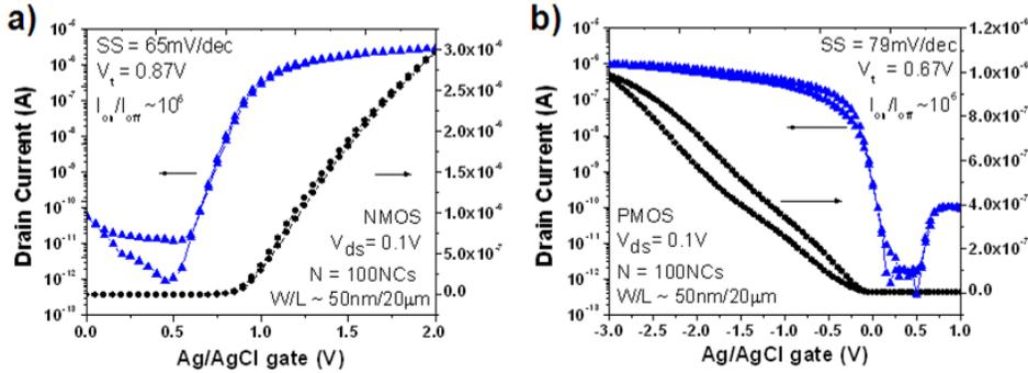
Figure 2: Transfer characteristics of (a) NMOS and (b) PMOS NG-FETs with 100 nanochannels (NCs)
