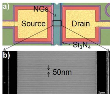
Figure 1: (a) Optical image of NG-FETs with 100 nano channels (b) SEM image of magnified area of multiple nanochannels ( $W=50\text{nm}$ ,  $t=30\text{nm}$ ,  $L=20\mu\text{m}$ ) connecting highly doped n or p-type source/drain pads.
