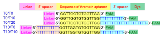
Figure 3: Design of the biomolecular probes examined in this study. They are denoted using the numbers of thymines ( N ) for 5' and 3' spacers as T0/T0.
