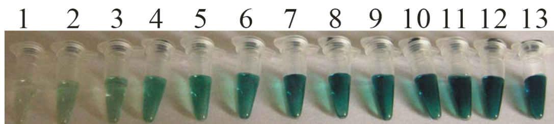
Figure S2. Oxidation of ABTS by \text{H}_2\text{O}_2 in presence of hemin and different concentration of AG4. 0, 0.1, 0.2, 0.3, 0.4, 0.5, 0.7, 0.9, 1.1, 1.3, 1.5, 1.7, 2.1 \mu\text{M} AG4
