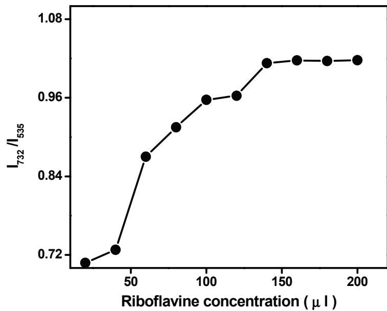
**Figure S3:** Ratio of peak intensity ( $I_{732} / I_{535}$ ) vs riboflavin concentration with same concentration of Au NPs and melamine (1  $\mu M$ ).
