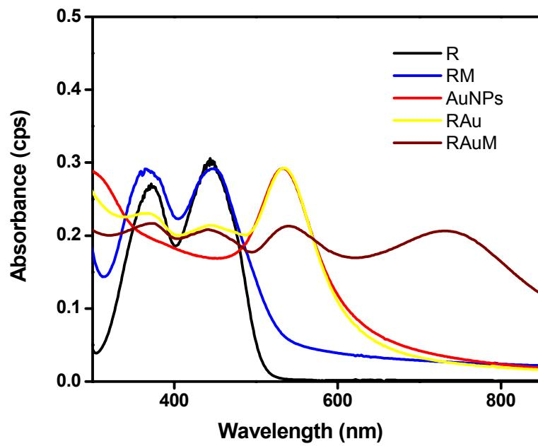
**Fig. S1:** UV-vis spectra of pure R, RM, Au NPs, R-Au NPs and melamine sensed R-Au NPs (RAuM).
