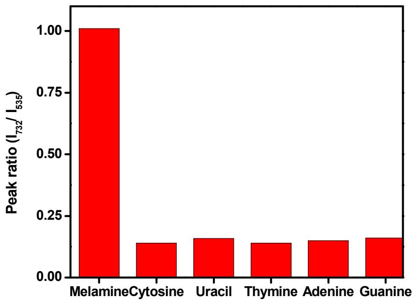
**Figure S4:** The selectivity of the optimized sensor for melamine in presence of different pyrimidine and purine molecules under similar condition.
