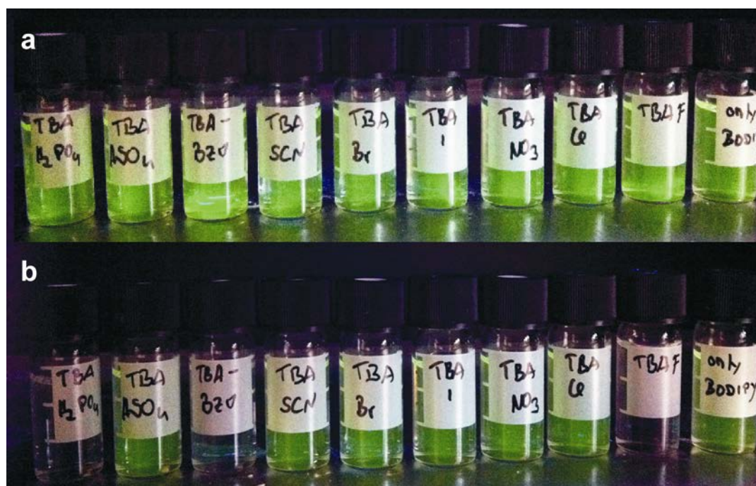
Figure S5. Visible response of 1 to various anions under UV-light a) in EtOH/H 2 O b) in MeCN.
