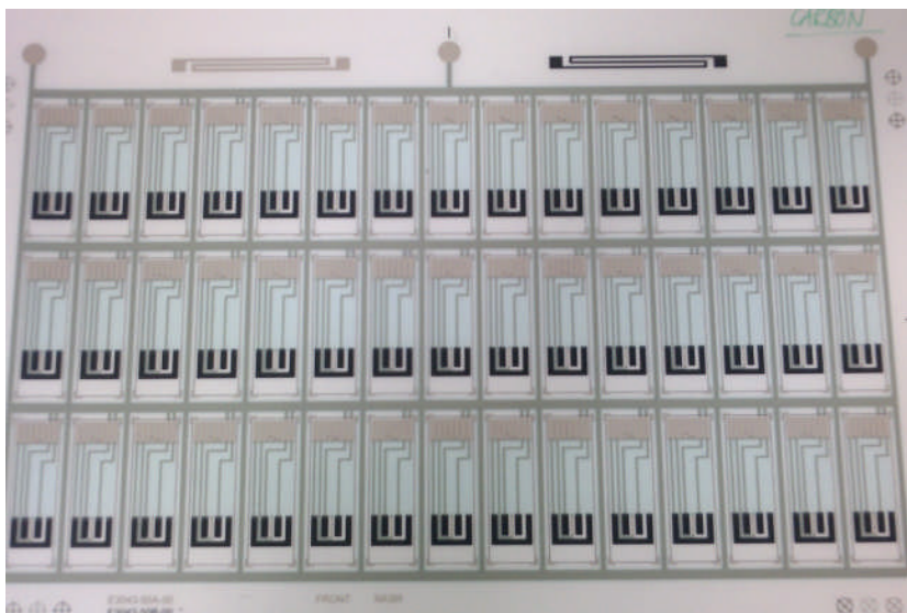
Figure S1 - A sheet of screen-printed carbon electrodes as received from Microarray (Manchester, UK)
