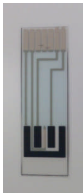
Figure S2 - An individual screen-printed sensor used in all electrochemical interrogations
