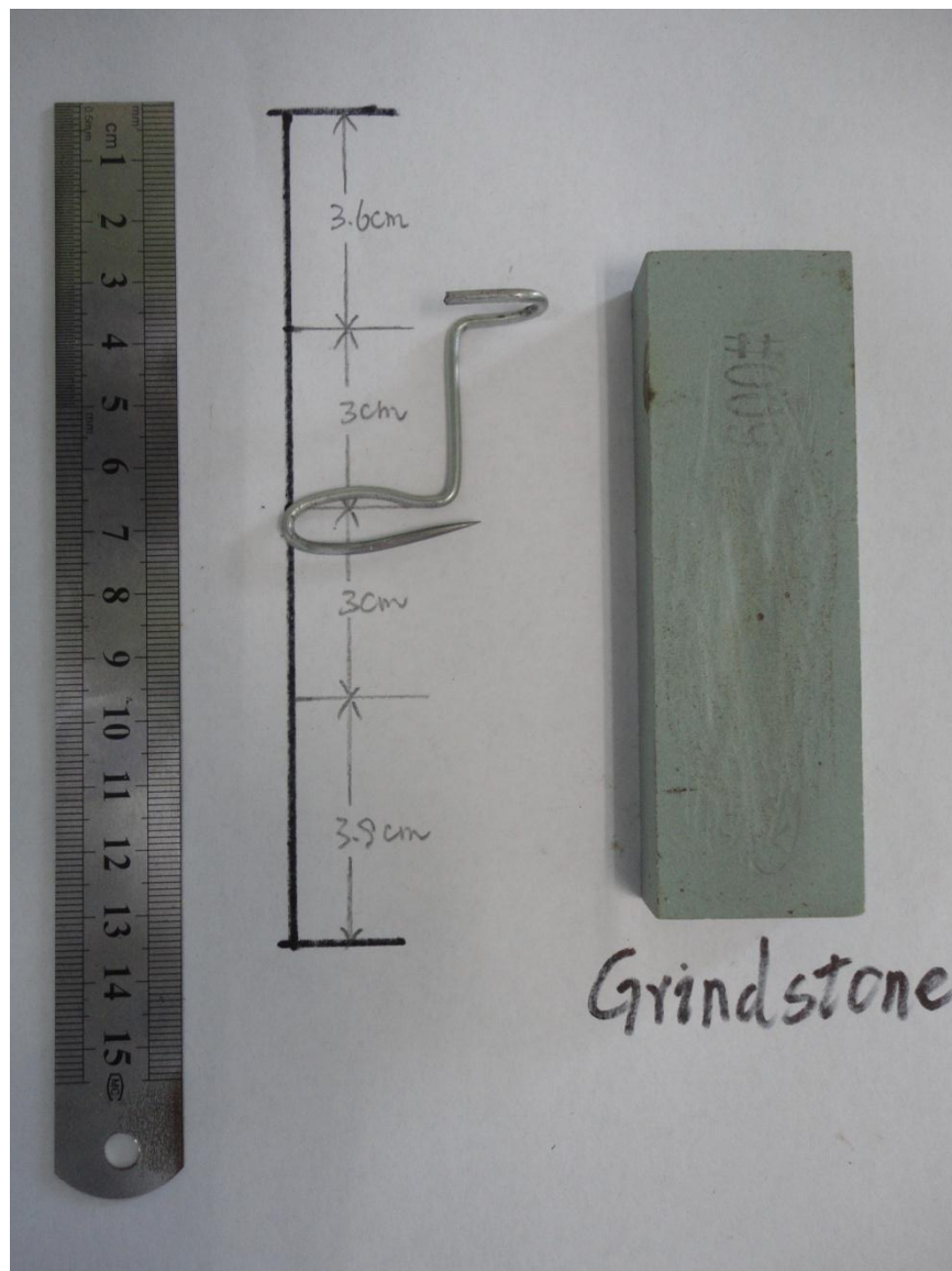
Fig S7. Grinding operation: use a grindstone to polish the tip.
