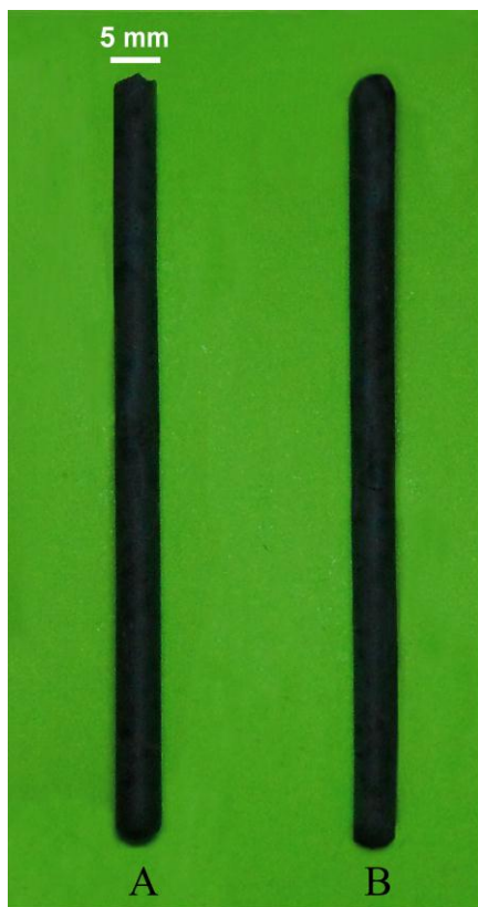
Figure S-1. Photograph images of OMAD-MMC with different MWNTs weight ratios: (A) 3 wt%, (B) 5 wt%.
