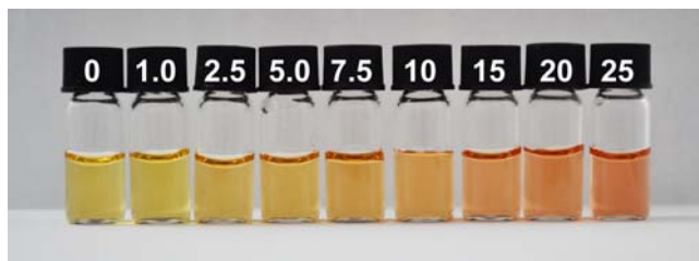
Fig. S2 Changes in the colour of PMTEMNa 2 ( 1.0 \times 10^{-4} M) solutions in the presence of increasing concentrations of paraquat as indicated ( \mu\text{M} ).
