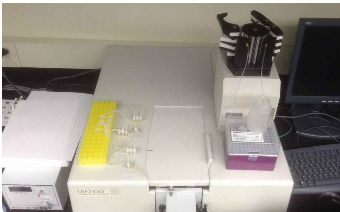
Figure ESI-2: The experimental setup. The photo shows the flow cells, spectrophotometer and peristaltic pump.
