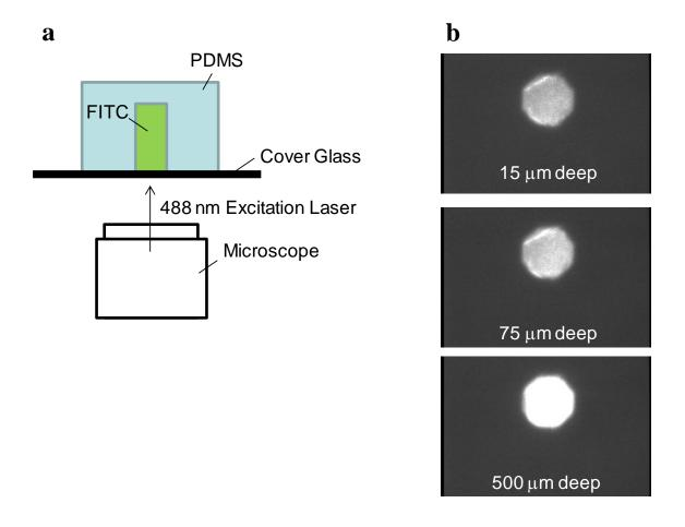
**Figure S-1:** Fluorescence experiment with deep PDMS microchannel. (a) Schematic illustration of the setup. (b) Obtained fluorescent images of 10 nM FITC solution.
