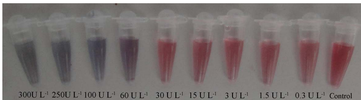
Fig. S1. The \beta -glucosidase concentration-dependent color changes. From left to right: 300 U L -1 ; 250 U L -1 ; 100 U L -1 ; 60 U L -1 ; 30 U L -1 ; 15 U L -1 ; 3 U L -1 ; 1.5 U L -1 ; 0.3 U L -1 ; Control sample.
