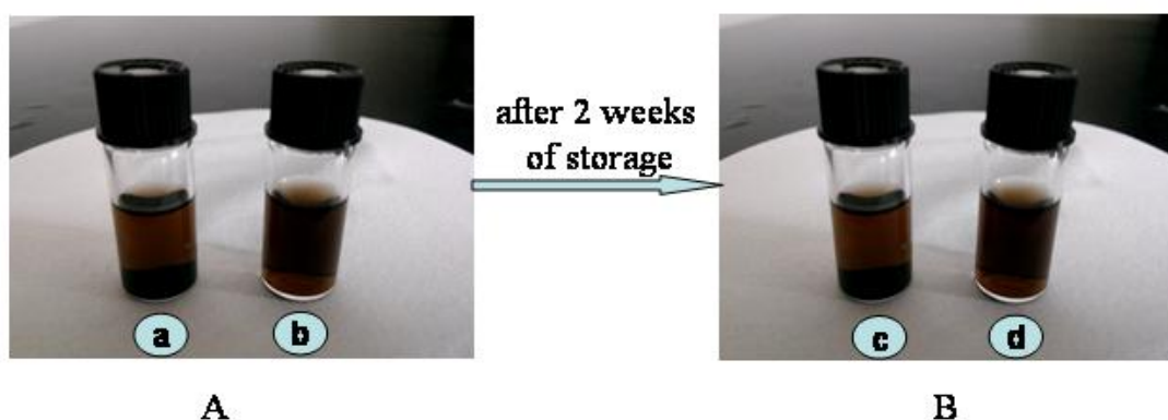
Fig.S1 Photographs of suspensions (A) new made, (B) after two weeks of storage of GO in water (a and c) and in the mixture of 1-propanol/1,4-butanediol (w/w=1/1) (c and d).
