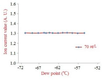
The detected signal of 70  $\mu$ g/L  $^{SO_2}$  from a standard solution is constant when the dew point of the scrubbed air flow was changed from -70 °C to -55 °C and the dew point of the total flow was raised to around -40 °C, which was measured in between the membrane filter and the FAIMS instrument shown in Fig. 2.
