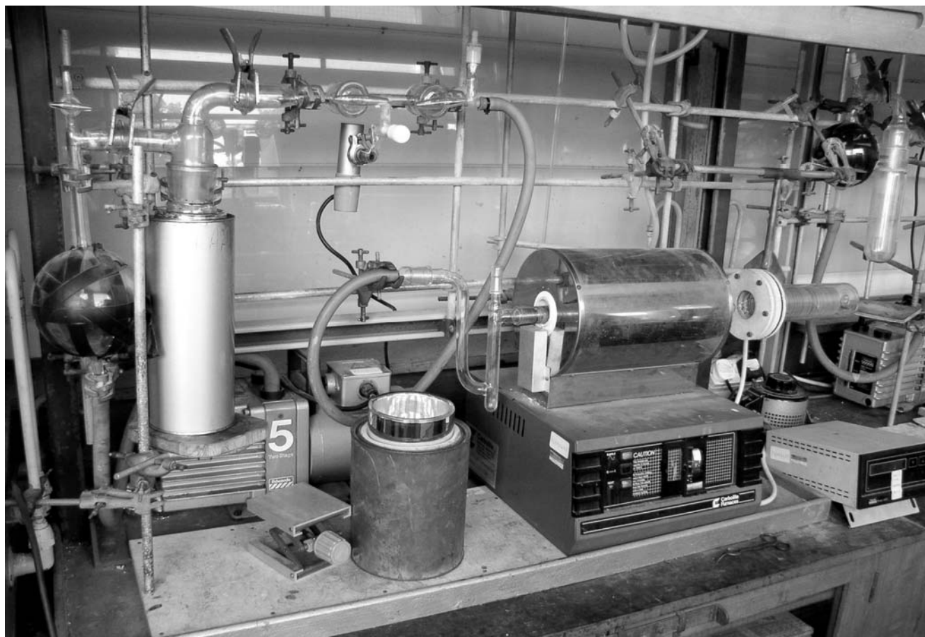
Figure SM 10.9.1: Photograph of FVP apparatus showing product collection trap
