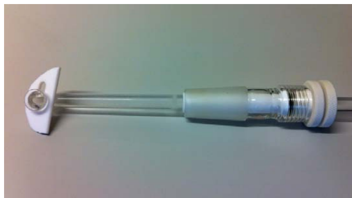
Figure SM 10.2.4. In order to secure fast and steady stirring a stirring rod with a bearing and a Teflon blade is used. Adequate equipment can be purchased for instance from Kontes, Vineland, NJ, USA.
