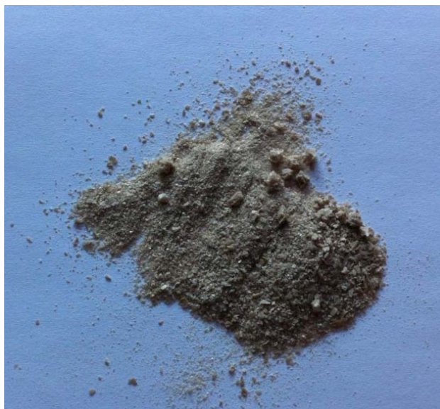
Figure SM 10.2.5. The product may get a brownish look or almost grey like here. When dried under vacuum at around 50 °C for some hours, the crystalline material may become a powder.
