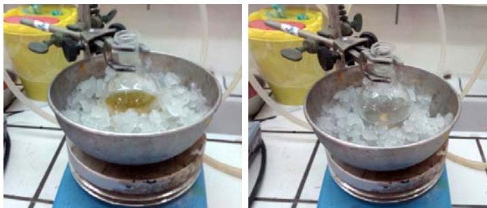
Figure SM 10.4.3. a) Step 1 at t=0 , 2-nitroaniline orange color; b) Step 1 at t=1\text{h} , colorless diazonium salt.
