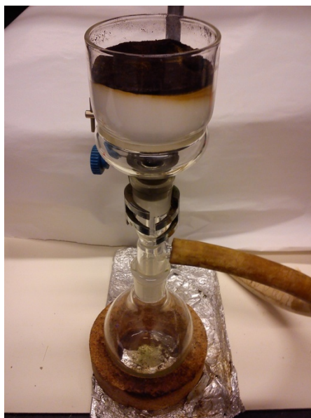
Figure SM 12.1.4.3. Silica filtration of the reaction mixture with a Buchner funnel.
