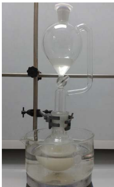
Figure SM 12.1.2.1 - Apparatus for oxidation of 1,2-tetradecanediol.
