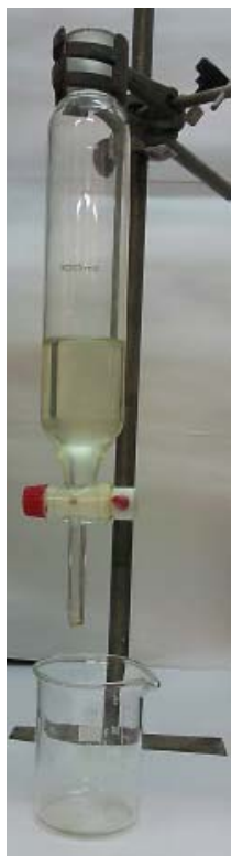
Figure SM 12.2.1.6 – Liquid-liquid extraction setup for the isolation of the product (laboratory session 1).
