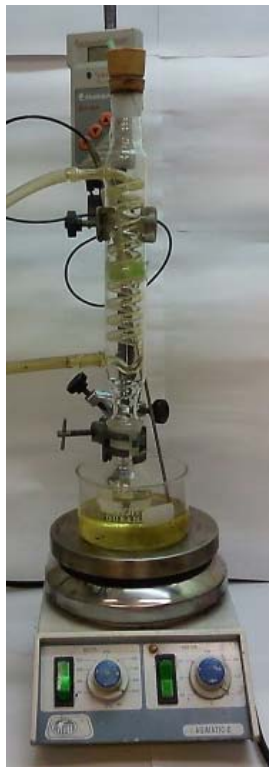
Figure SM 12.2.1.5 – Reaction setup for the intramolecular oxidative cyclisation reaction (laboratory session 1).
