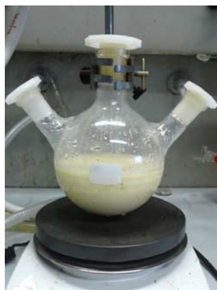
Figure SM 12.2.5.4 – Visual aspect of Reaction 2 after 4 hours at 70°C (the thermometer was removed).
