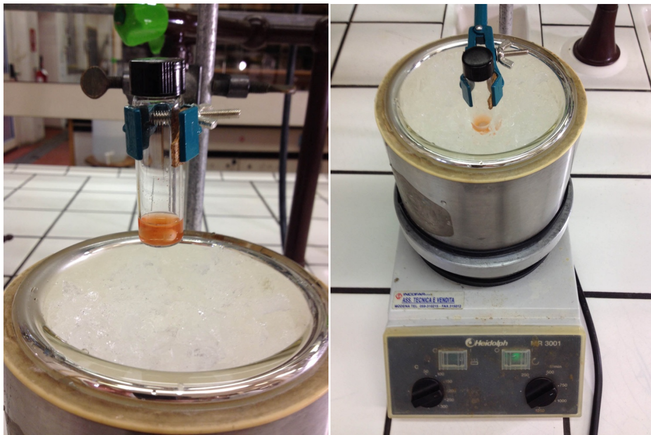
Figure SM 2.2.4.7 – Setup of the experimental apparatus for organocatalytic alkylation of aldehyde.
