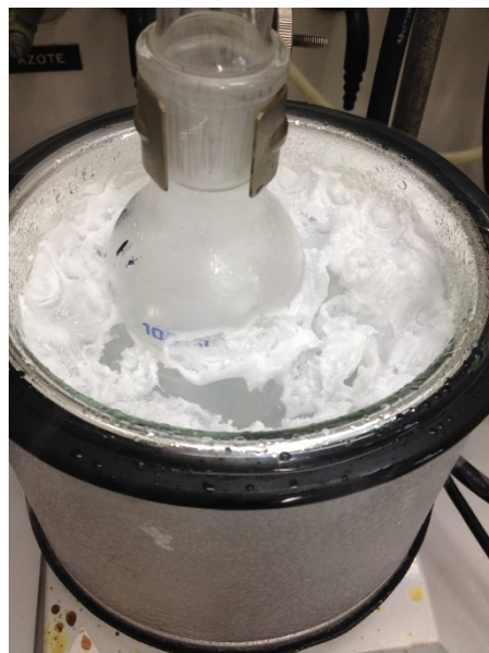
Figure Error! Not a valid bookmark self-reference.1 –Methanol bath cooling at -98°C
