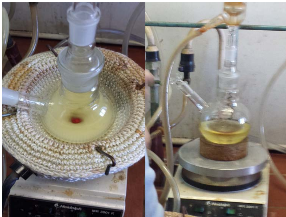
Figure SM 2.2.1.1. Mixture of 3-methyl-1-phenyl-1H-pyrazol-5-one and \text{Ca}(\text{OH})_2 before (left) and after (right) heating.
