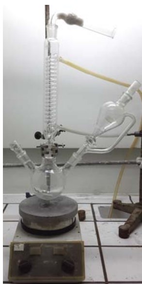
Figure SM 3.2.3.1 – Reaction set-up apparatus for dimedone
