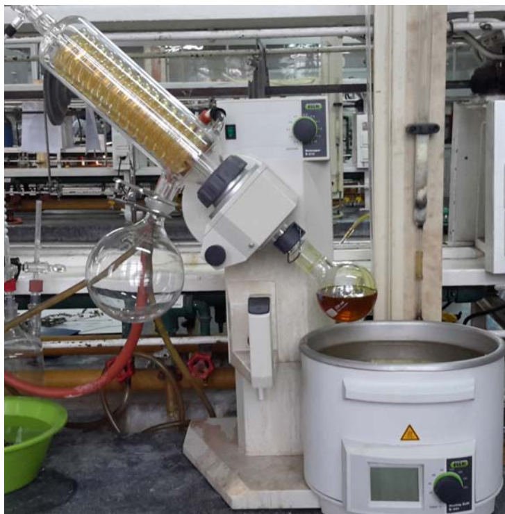
Figure SM 3.2.3.2 – Rotary evaporator for distillation of ethanol-water mixture
