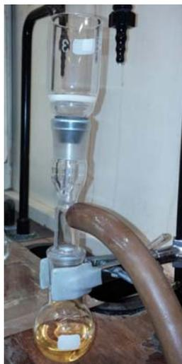
Figure SM 4.2.5.3.2. Reaction mixture filtration setup after the Ugi reaction.
