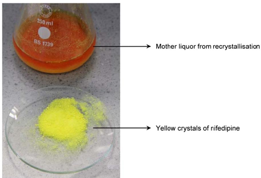
**Figure SM 4.2.5.2.2** – Nifedipine after recrystallisation and filtration (student sample).
