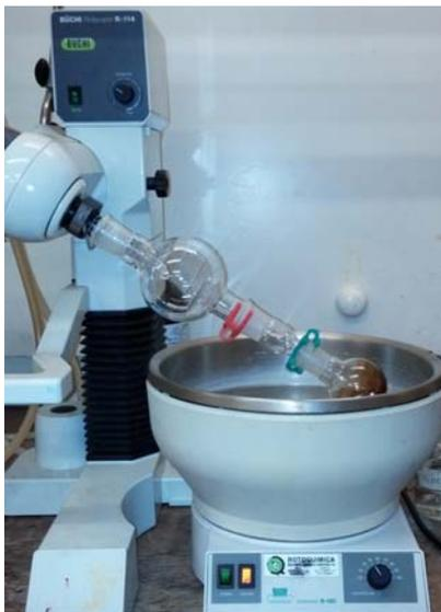
Figure SM 4.2.5.3.3. Rotary evaporation of solvent from reaction mixture.
