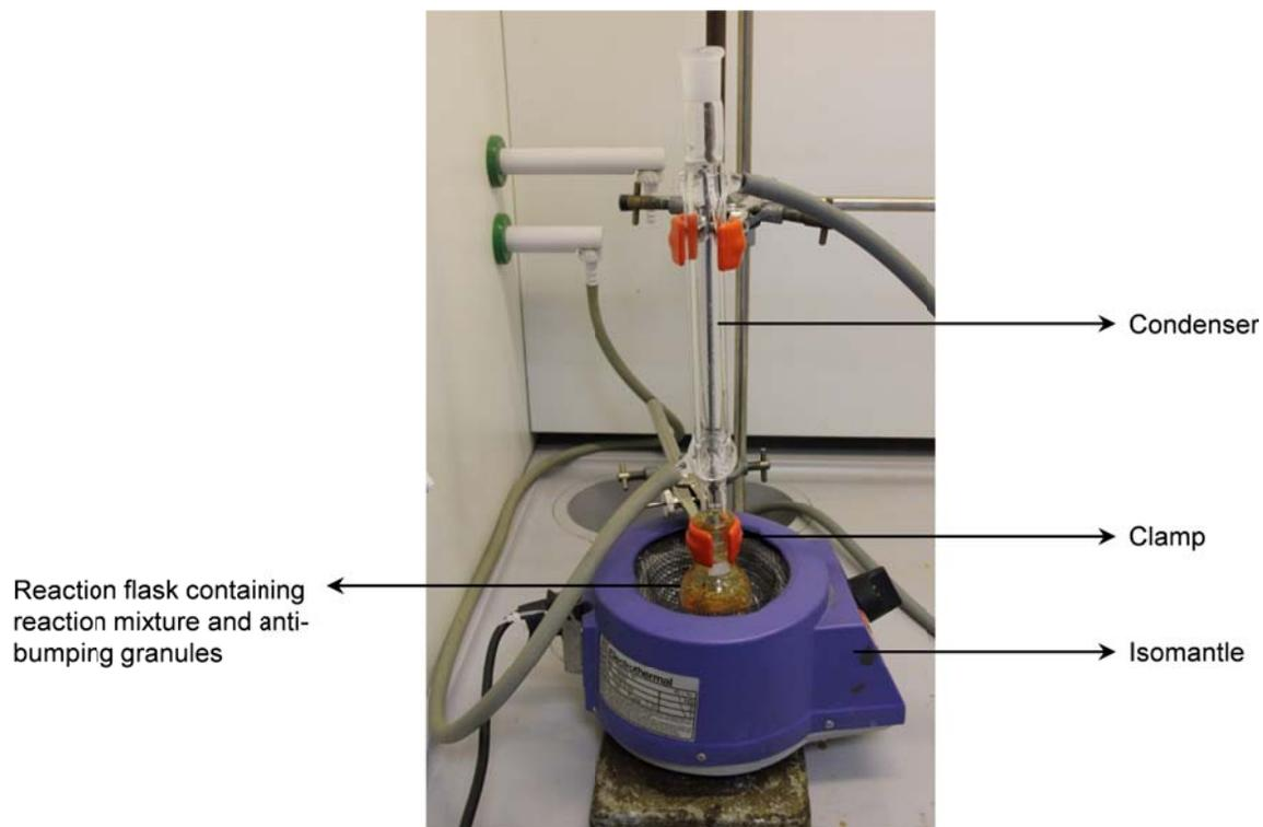
**Figure SM 4.2.5.2.1** – Reaction mixture during the reflux step. Formation of nifedipine is evident from the yellow-orange colour of the solution.
