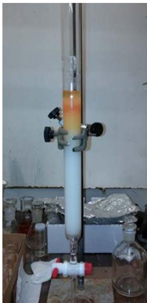
Figure SM 4.2.5.3.4. Column chromatography purification of the evaporated crude residue.
