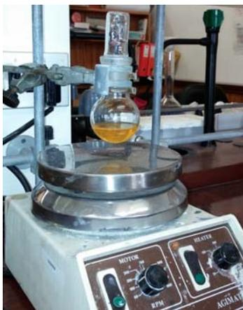
Figure SM 4.2.5.3.1. Reaction setup for the Ugi reaction.
