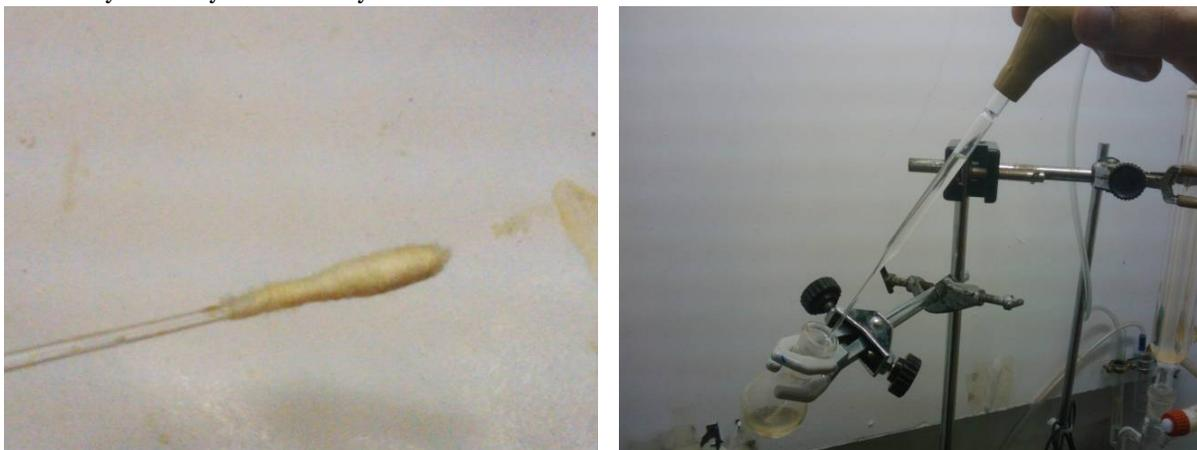
**Figure SM 4.2.5.4.1** - Filtration over cotton aided by Pasteur Pipette
