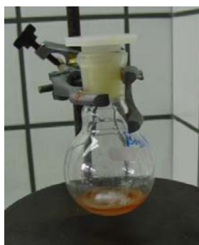
Figure SM 9.2.3.1 - Reaction mixture at time 0, 30 minutes and at the end of reaction. Note the red-brownish color gradually fading along the time
