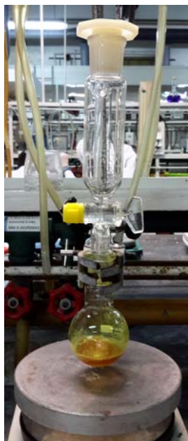
Scheme SM 9.2.1.1 – Reaction set-up apparatus for trans -9-(2-phenylethenyl)anthracene preparation.
