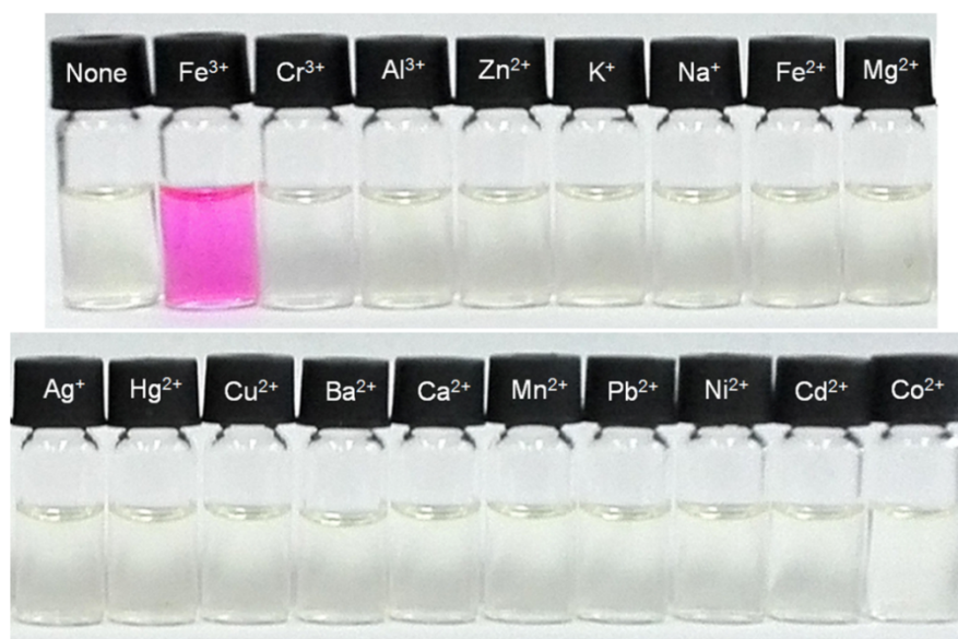
Figure S1. Color responses of RH-Fe (20 μM) in the presence of various metal ions (200 μM).
