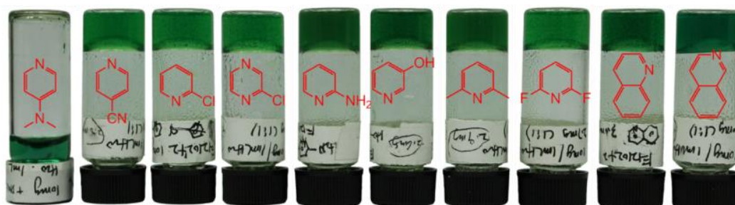
Figure S1. Collapsed sol and hydrogels formed by metallo gel 1a /H 2 O (1.0 wt%) with various additional pyridine derivatives.
